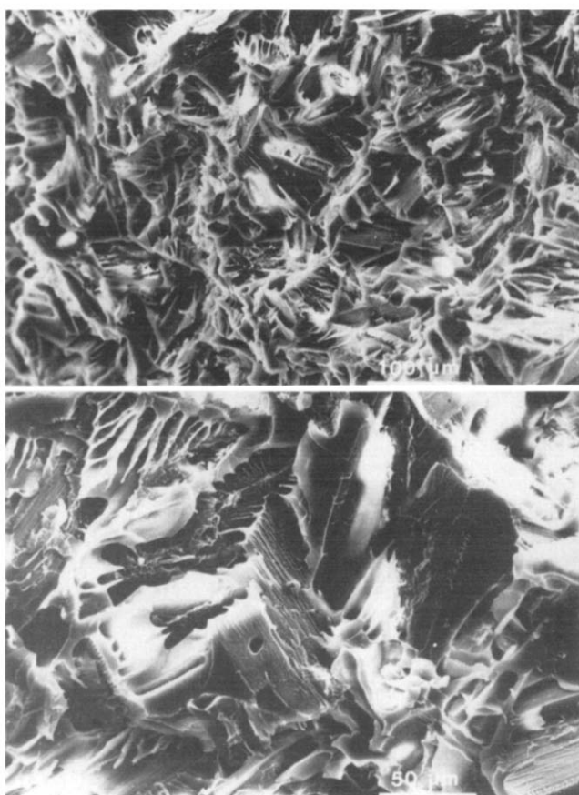
Figure 14 Scanning electron micrograph of the polymeric structure formed on solidification of the PLLA 60-HMB 40 (%w/w) mixture, which is close to the eutectic composition
